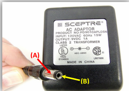
Figure 15.40. The barrel plug conductors from this wall transformer are labeled (A) and (B).
